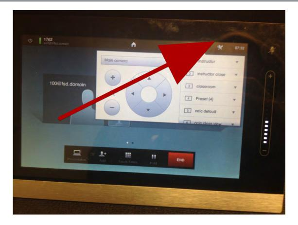
Select any of the preset views or use the arrow buttons to adjust the camera, or use the +/- to zoom the camera.
